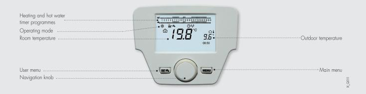
The "User menu" button provides direct access to basic settings such as: establishing temperature set points, operating mode (heating mode, heating set point, forced DHW mode, DHW set point, operating mode, etc.)
