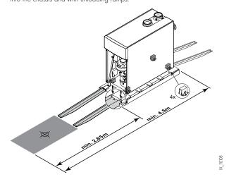
IX 245... boilers are equipped with lifting rings to facilitate installing the boiler.
