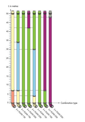
L max as a function of duct  $\ensuremath{\mathcal{O}}$  D, for various "cascade" combinations
