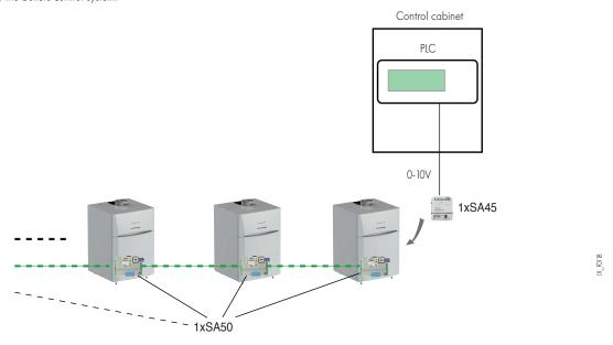
• Each boiler has a 0-10V connection by means of the MEWM control module (package SA45) to the PLC in the boiler room. It is the PLC which will manage the cascade, as well as all the secondary circuits.
